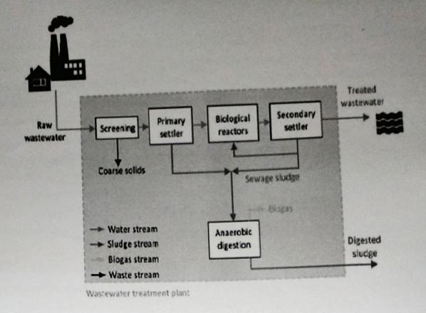
The physical process: this is the mechanical treatment of the water that involves removal of debris from the raw wastewater right from the point it enters the plant. The screening and primary settling of debris. Wastewater enters the treatment plant through the inlet chamber from where it is channeled to the coarse screen that removes solid waste.
